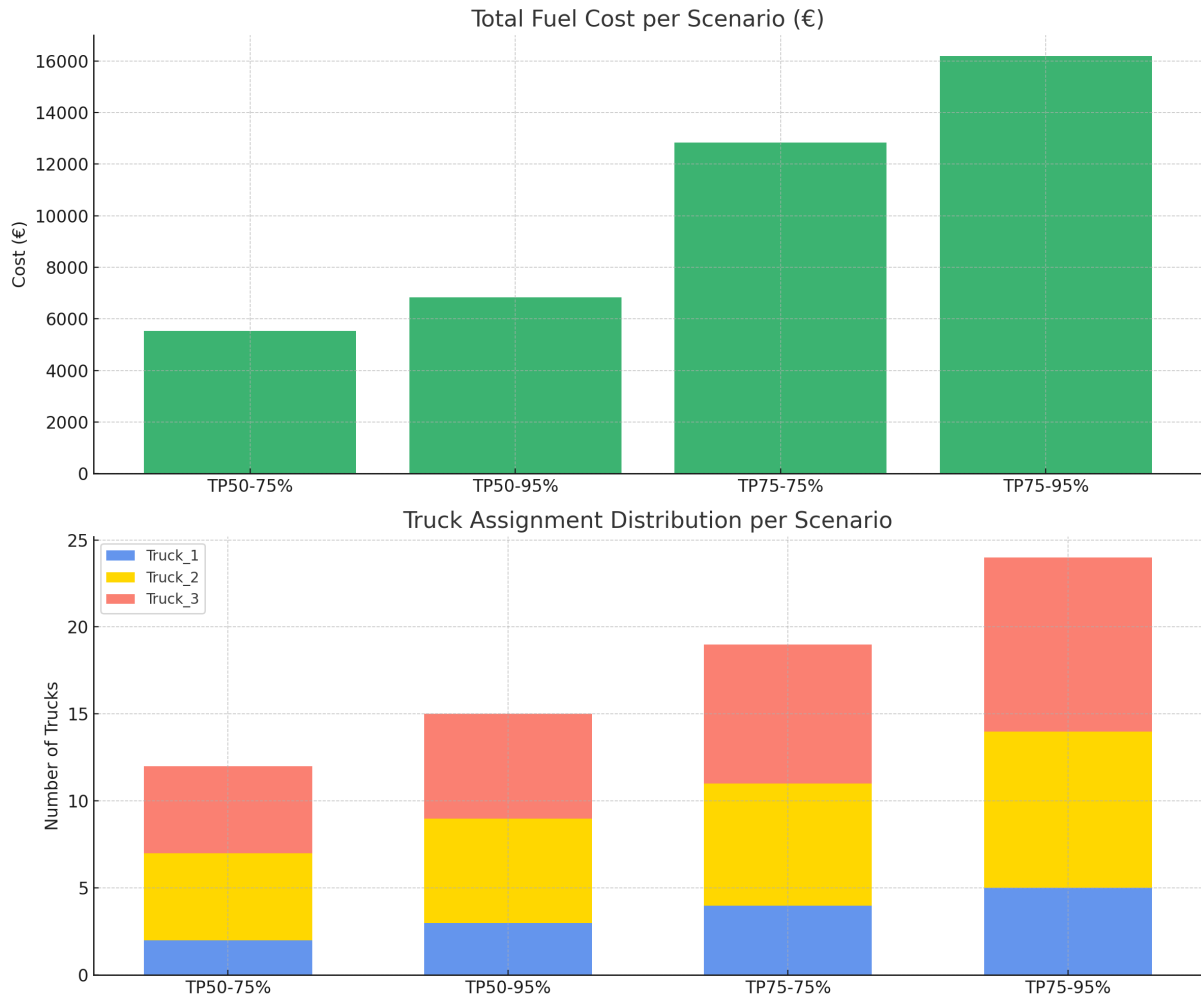
Figure 2.18: Truck assignment and fuel costs per scenario.
