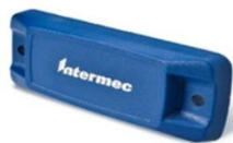
Figure 1 - RFID passive tag
