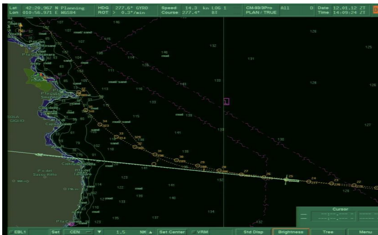
Figure 4. Overview of the navigation route prior to collision with the underwater rock (obtained by simulation)
